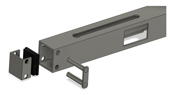
Two sections of 6mm dia steel bar, each 35mm long are welded 19mm apart into a small spacer cut from 2mm thick steel plate. The takedown clip is retained via friction.
