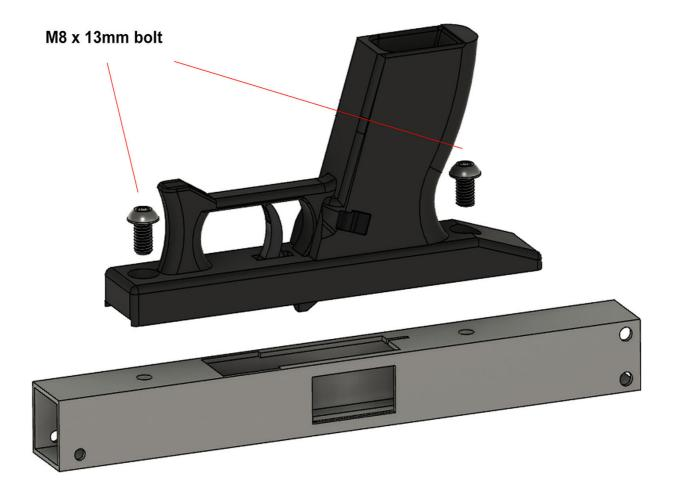
For the purposes of ease of construction each take-down bolt is threaded directly into the upper receiver tube. Upon final assembly loctite should be applied. Alternatively two M8 nuts can be welded to the receiver and the lower receiver body drilled using a 13mm bit to accommodate each.
