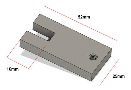
2mm steel plate. Weld in place.
