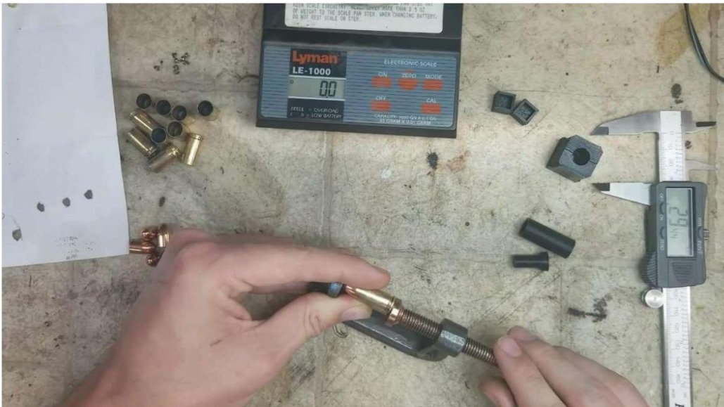
Step 5: Seating bullet into case.
