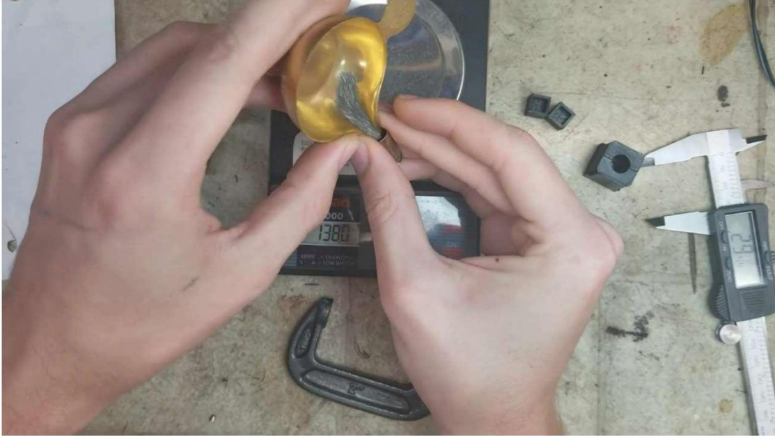
Step 3: Dumping 3.5gr of powder into the case.
