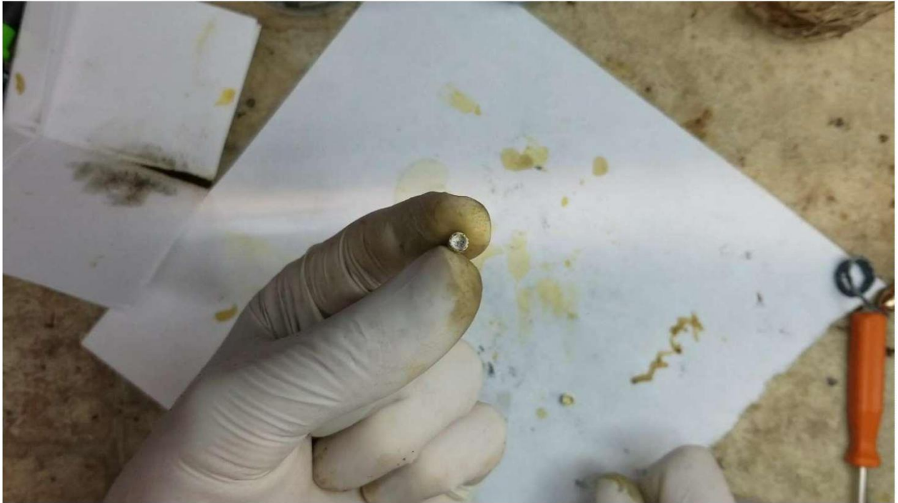
Step 8: Primer compound compacted; paper disc pressed down into the cup.
