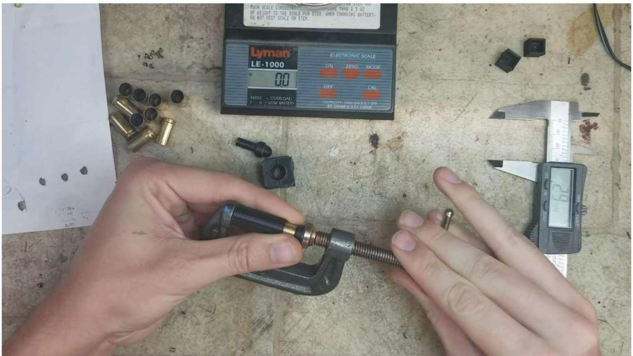
Step 1: Pressing a primer into place
