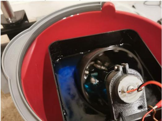
Be careful not to overfill the drum. Bullets should not fly out or make the drum hard to rotate. Connect the Anode (copper donor) to the positive terminal of your PSU, and connect the Cathode
