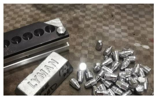
Once you have a sufficient number of bullets cast, you are now ready to electroplate or powder coat your lead bullets.
