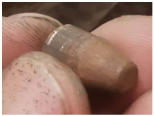
If the bullet engages the rifling well and does not shed copper, you've done an excellent job. You can load them into 9mm cartridges now. Follow the instructions provided by Ivan in BWA volume I to reload cartridges. I recommend you weigh the bullets first and find the average weight of the batch. It will be helpful for you to determine the amount of propellant for reloading.
