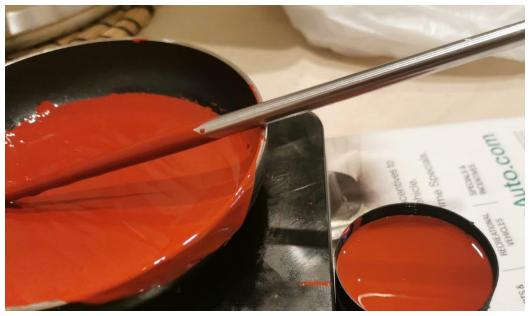
Next, flick the mold for about a minute to assist the bubbles escaping. Bubbles trapped will cause defective casts.
