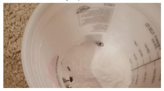
Your bullets should pick up an even layer of powder now. Carefully remove the bullets using a soup spoon with holes and place them on the toaster oven tray.
