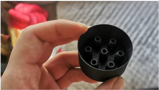
Mix the silicone in a container with a pair of chopsticks. The silicone and curing agent should have a weight ratio of 100:3. Pour the well-mixed silicone into the 3d printed bullet mold slowly and steadily to avoid bubble formations. If you have hollow-point bullets, dab a little bit of silicone with your chopsticks to fill up the tip of the hollow point first to avoid bubble build up.
