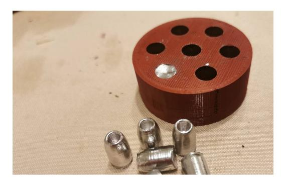
After the bullets cool down completely, you can acid soak them and throw them into the electroplating machine following the guide in part 2. Beware the bullet diameter is intentionally undersized by 100um to make sure thick enough copper can be plated. You will have to leave the plating machine running longer and check a few bullets' diameters every few hours.
