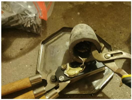
Wait for about 30s for the lead to solidify, then shear off the extra lead using the outermost handle of the mold. The additional lead sheared off can be put back into the crucible.
