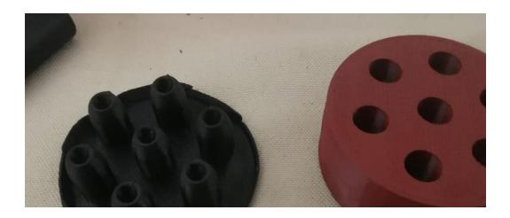
After inspecting your newly made silicone mold, you can then melt some lead and pour it into the mold like in part 1. However, the silicone cannot withstand anything hotter than 300C, which is about the melting point of lead. You have to control your pour temperature very carefully or you will damage the silicone. A thermometer is recommended.
