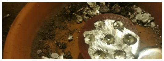
Unlike the metallic LEE mold, the silicone does an absolutely terrible job dissipating heat. Leave your silicone mold to cool down for a few minutes before you remove the freshly cast bullets. The mold is ready to be used again. I have used the silicone mold over 15 pours, and the mold has experienced no visible damage, and the bullet dimension remains consistent.
