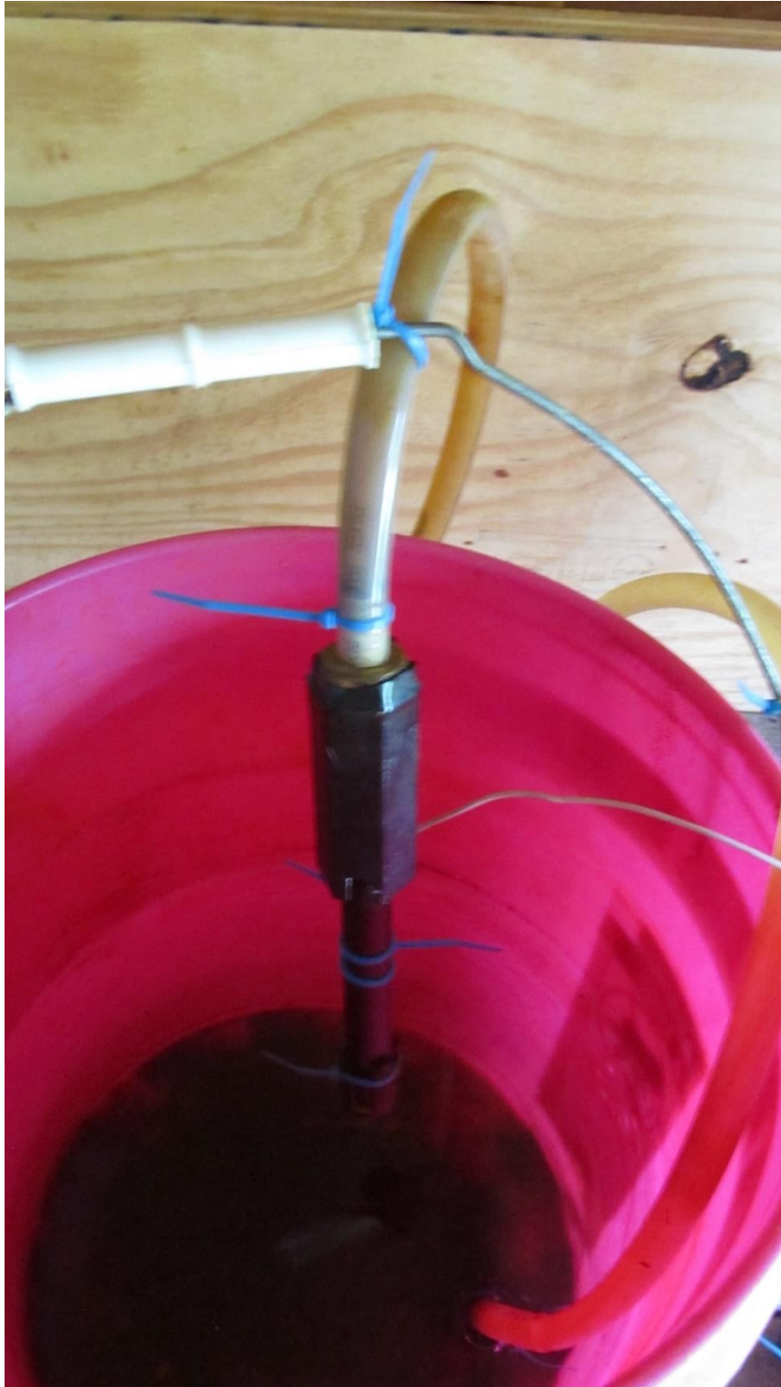
Step 17 continued: MOUNTING THE TOOLHEAD – example picture showing the toolhead hanging above the bucket. Note position of zip ties.
