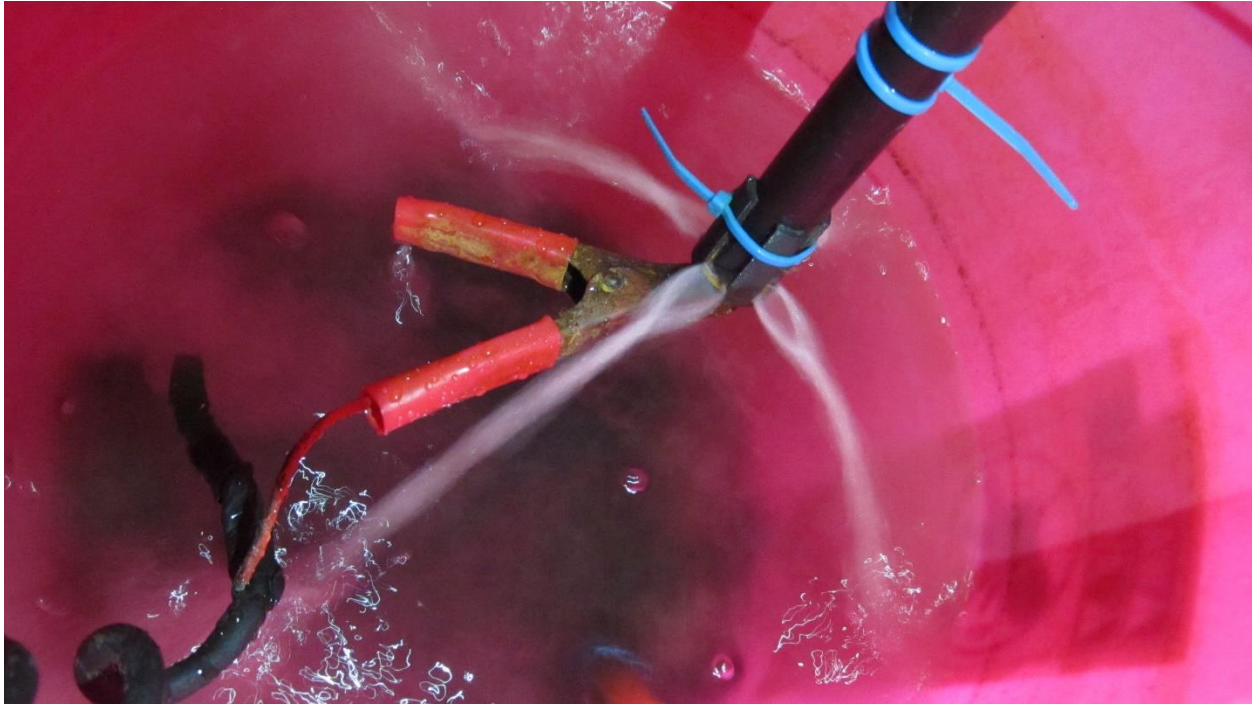
Step 19 continued: BORING OPERATION – Example of the lighter color of the fluid once the power supply is turned on. A hissing sound may also be heard.
