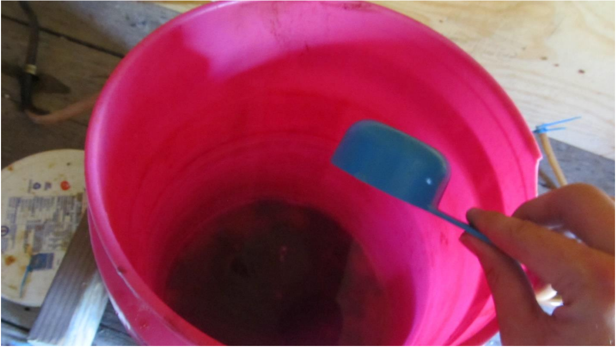
Step 3: PREPARING ELECTROLYTE - Pour your salt into the reservoir. Mix it in.
