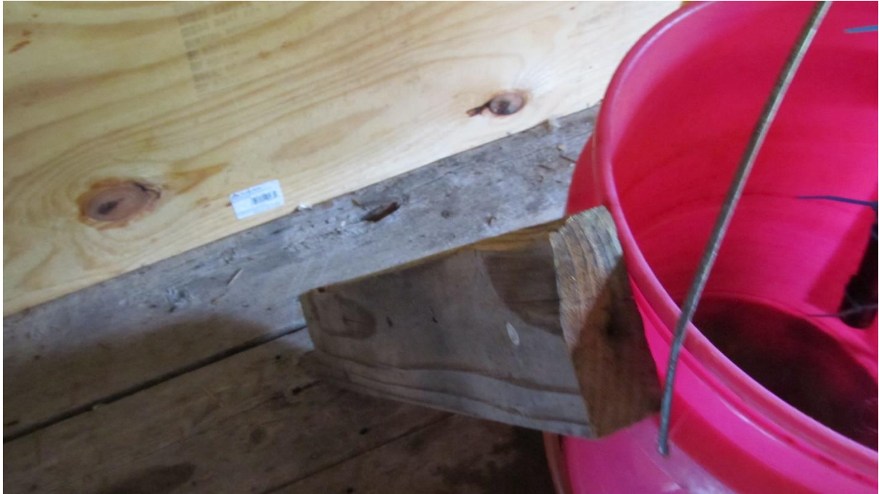
Step 17 continued: MOUNTING THE TOOLHEAD – Example picture showing using a block of wood (2x4) to prop up the handle of the bucket to hang the toolhead above the bucket.
