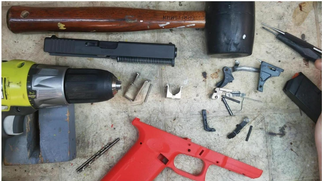
Spread of parts and tools used in assembling a DD17.2 Glock Frame
