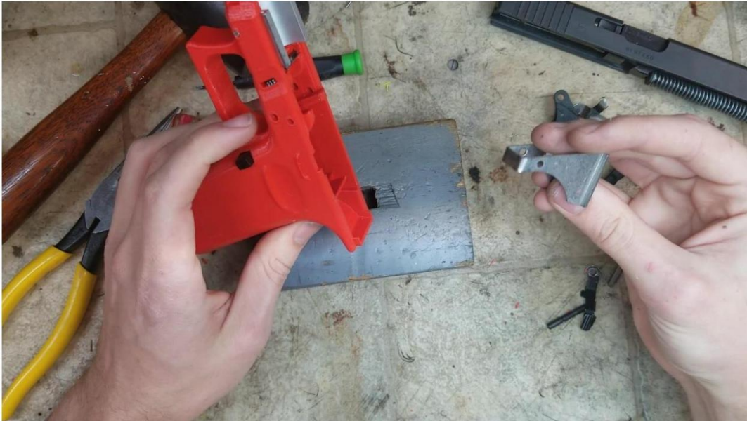
Orientation to install the rear rail. The curved side goes to the rear of the frame. The longer rail edge goes on the left hand side.
