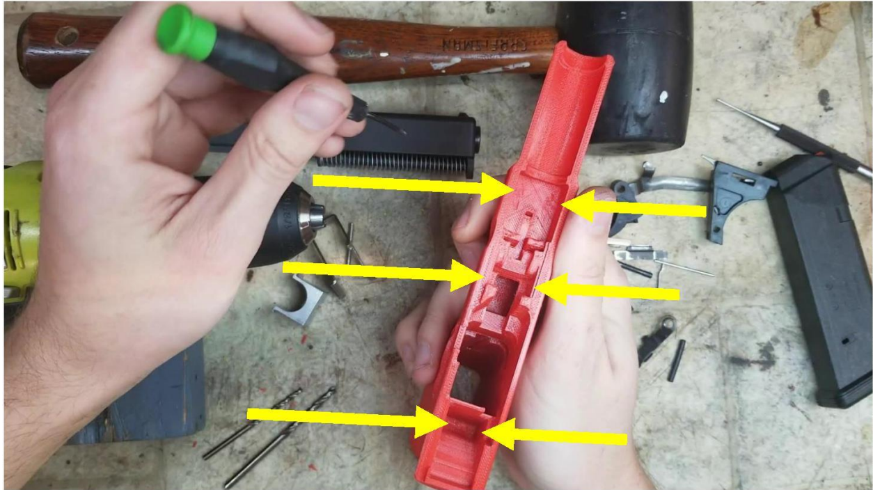
View of all three pockets needing close attention, as well as a suitable screwdriver to remove stubborn supports. The six arrows indicate the areas where stubborn support material may remain. Get it all out.
