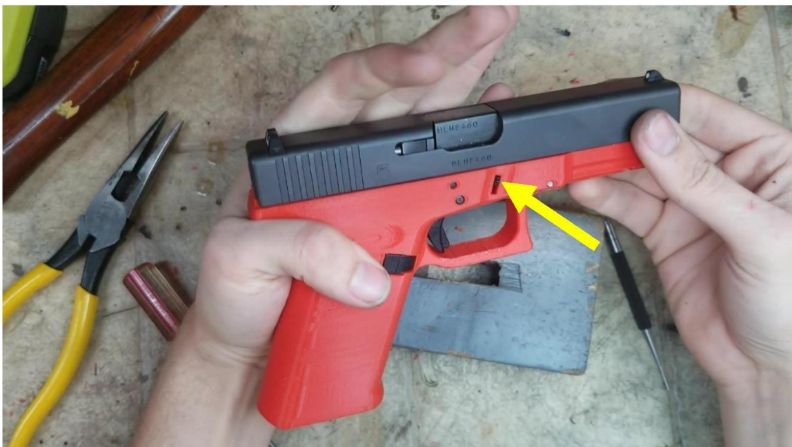
Slide installed. The slide latch should pop up after the slide is fully pushed back.
