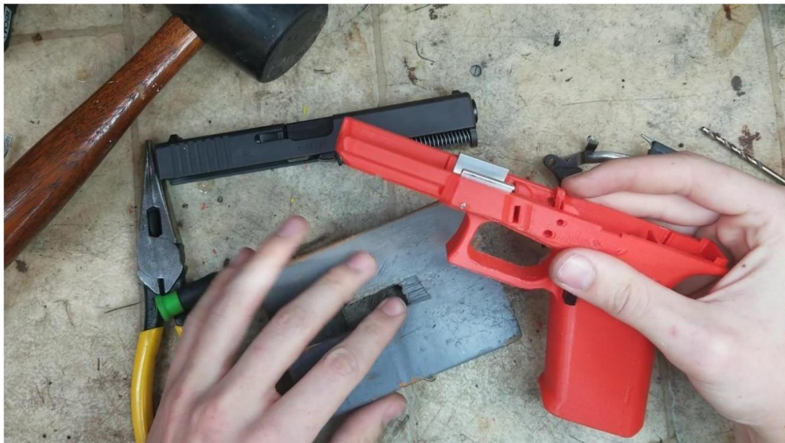
Front rail pin installed. You may need to use a hammer and punch.
