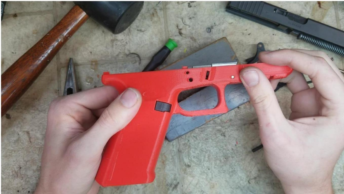
Locking block fully inserted. The holes should line up.
