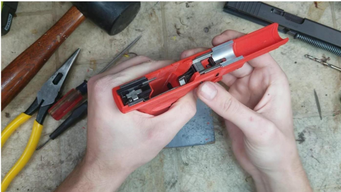
Push the pin all the way into the frame. It should sit evenly inside the frame.
