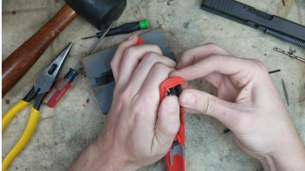
Push the rail and trigger block down firmly. The trigger bar and trigger should naturally fall into the frame.
