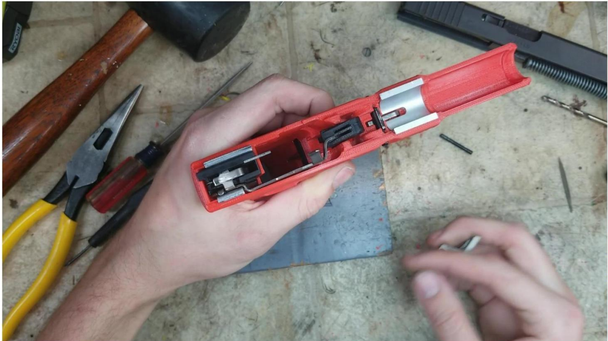
Trigger sitting inside the pocket as it should.
