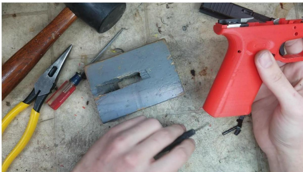
Check pin hole alignment. Try to wiggle things around to make them line up. Drill if needed.
