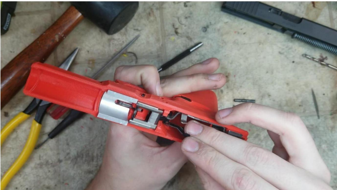
The slide stop being place between the trigger and frame
