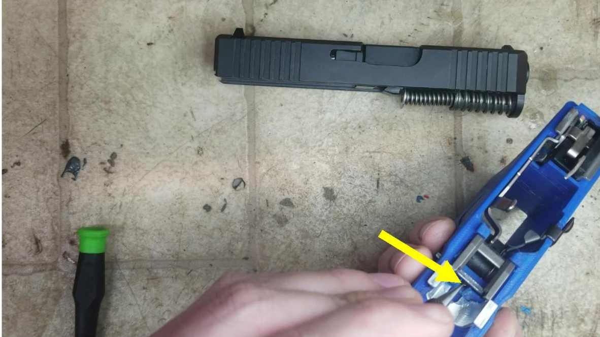
Push down on the spring from this slot in front of the slide latch. Push the latch down a hair and out the side.
