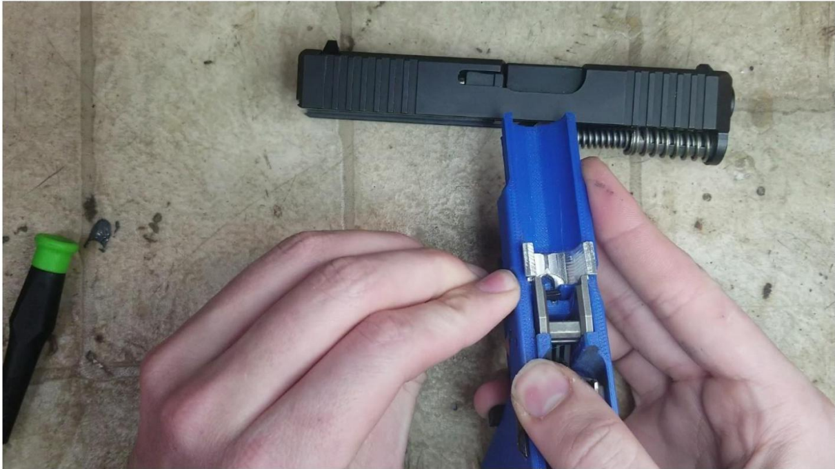
Pushing down spring with the latch
