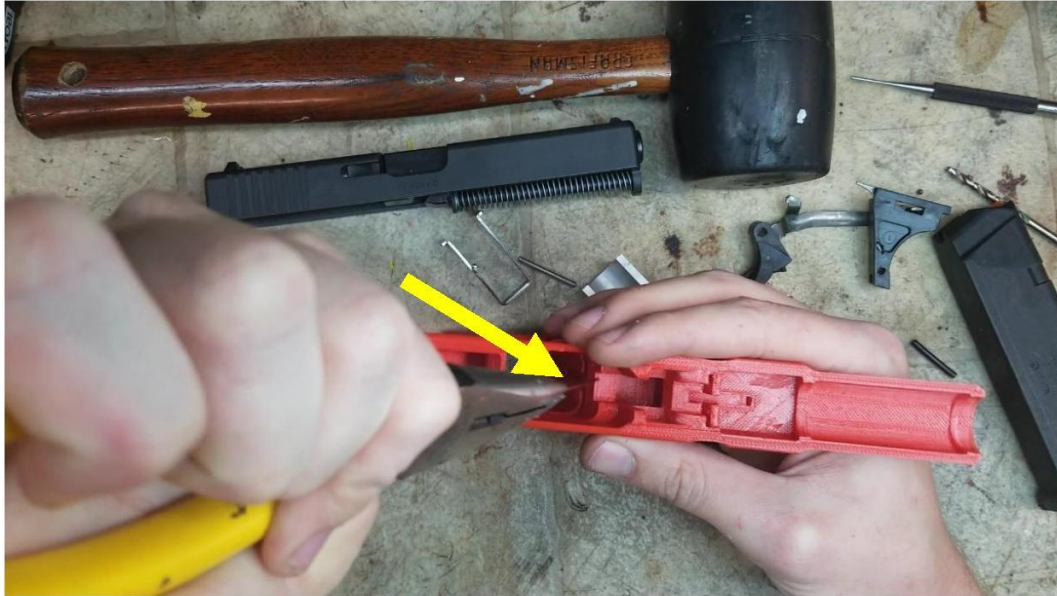
Installing the mag catch spring. The hole is located where the arrow points.
