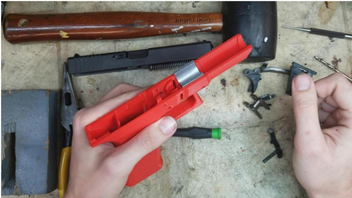
Front rail block placed in frame
