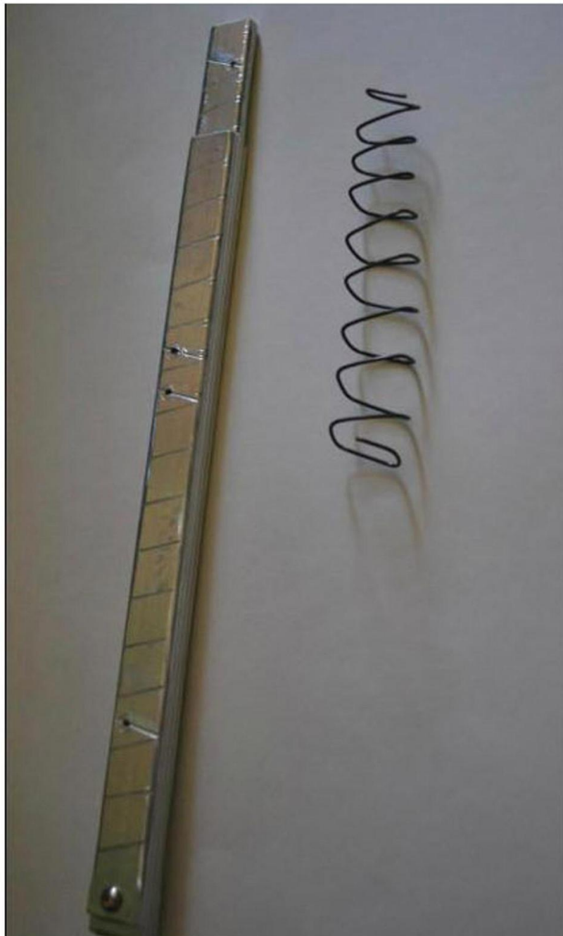
Spring winding jig and completed magazine spring.
