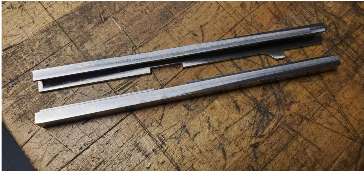
Example of milled spec Plastikov rails
