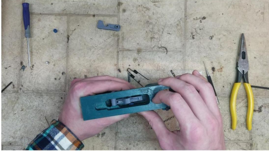
With a little practice, you can drop the whole trigger assembly into the receiver in one step
