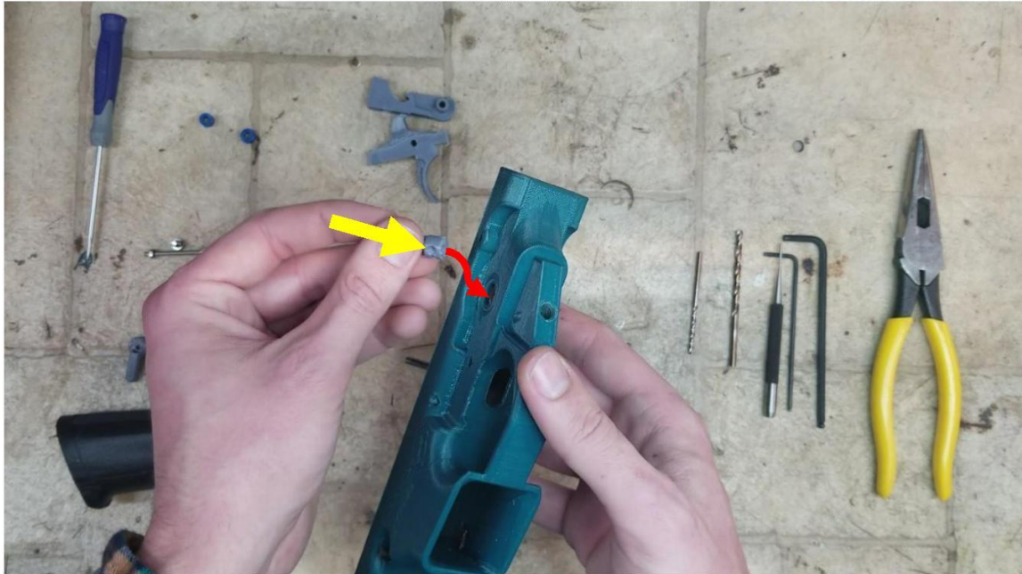
The drum should be installed so that the round detent cutouts in the selector should be on the right
