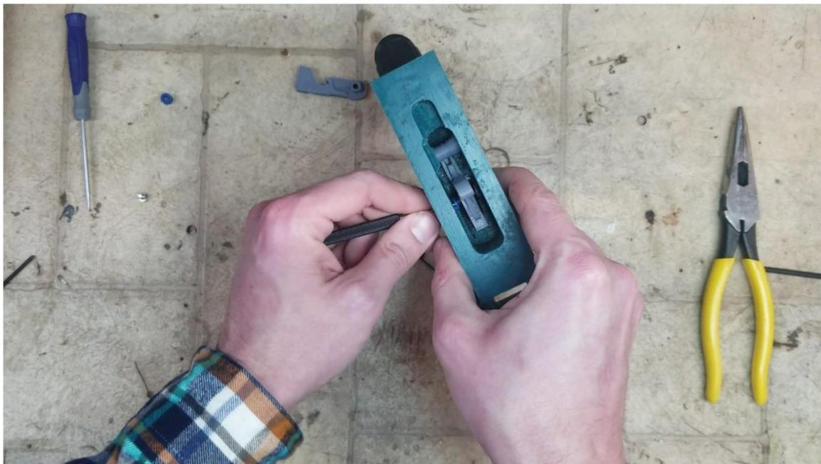
You can use a punch or screwdriver to help line up all of the pin holes while you push the pin through
