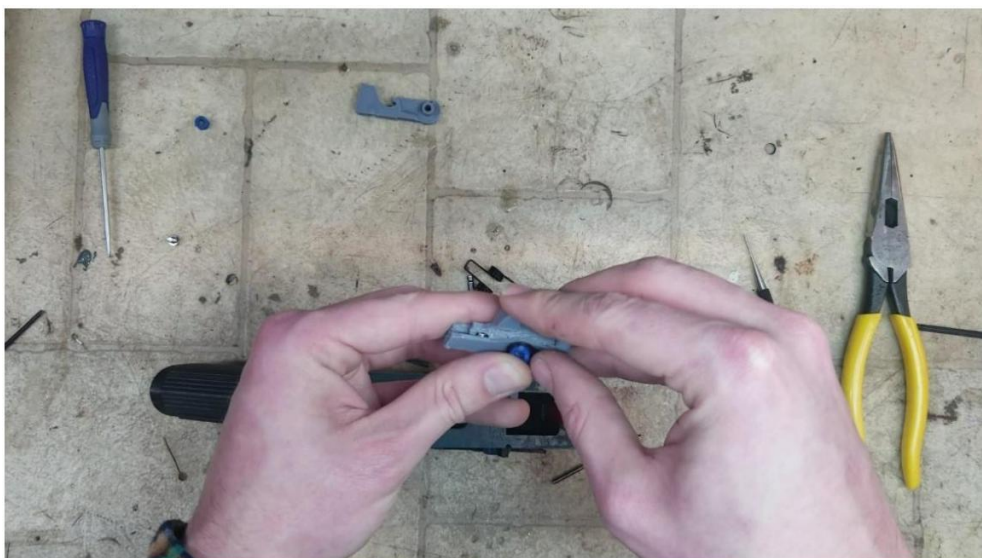
Install the trigger, trigger stud, trigger spring, disconnecter, and disconnecter spring as one unit
