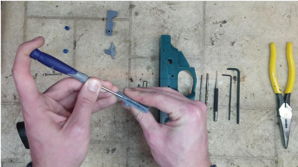
You can use a 3mm screwdriver to scrape the supports out of the channel inside the trigger.
