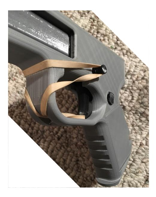
If you have a small rubber band for the trigger band, you can push one side through the front hole in the trigger guard and loop it around the trigger notch like before, but then take the other side and attach it to the trigger notch as well but without tucking it through the front trigger guard hole.
