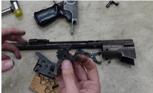
Take your trigger and disconnecter chassis.
