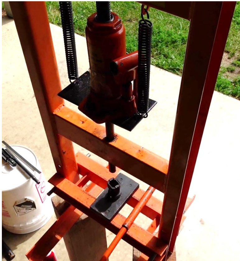
Position the trunnion like shown for pressing – the rear end of the trunnion should face up!
