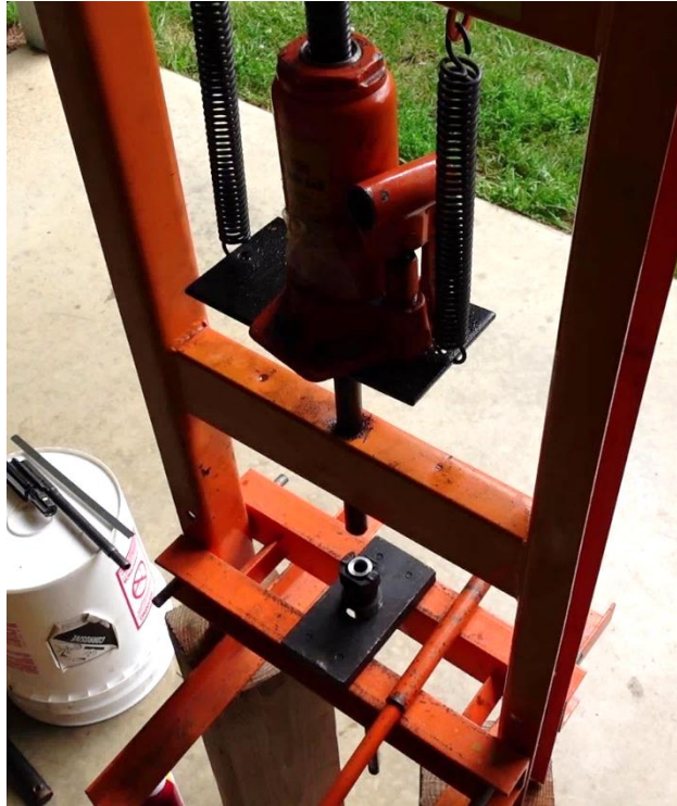
Place the barrel and trunnion together under the press ram.
