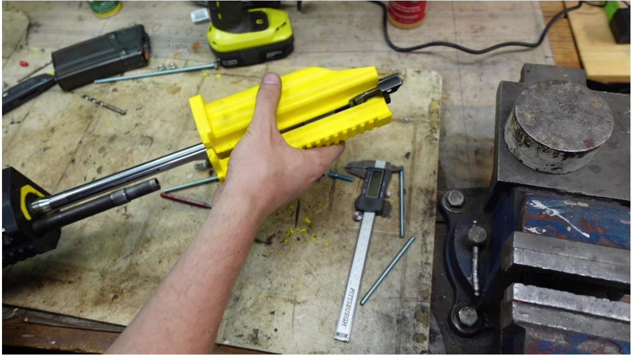
Slide the handguard over the barrel.
