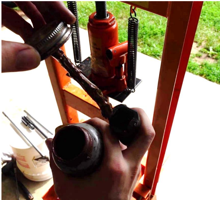
Apply a little grease to the barrel channel in the trunnion.
