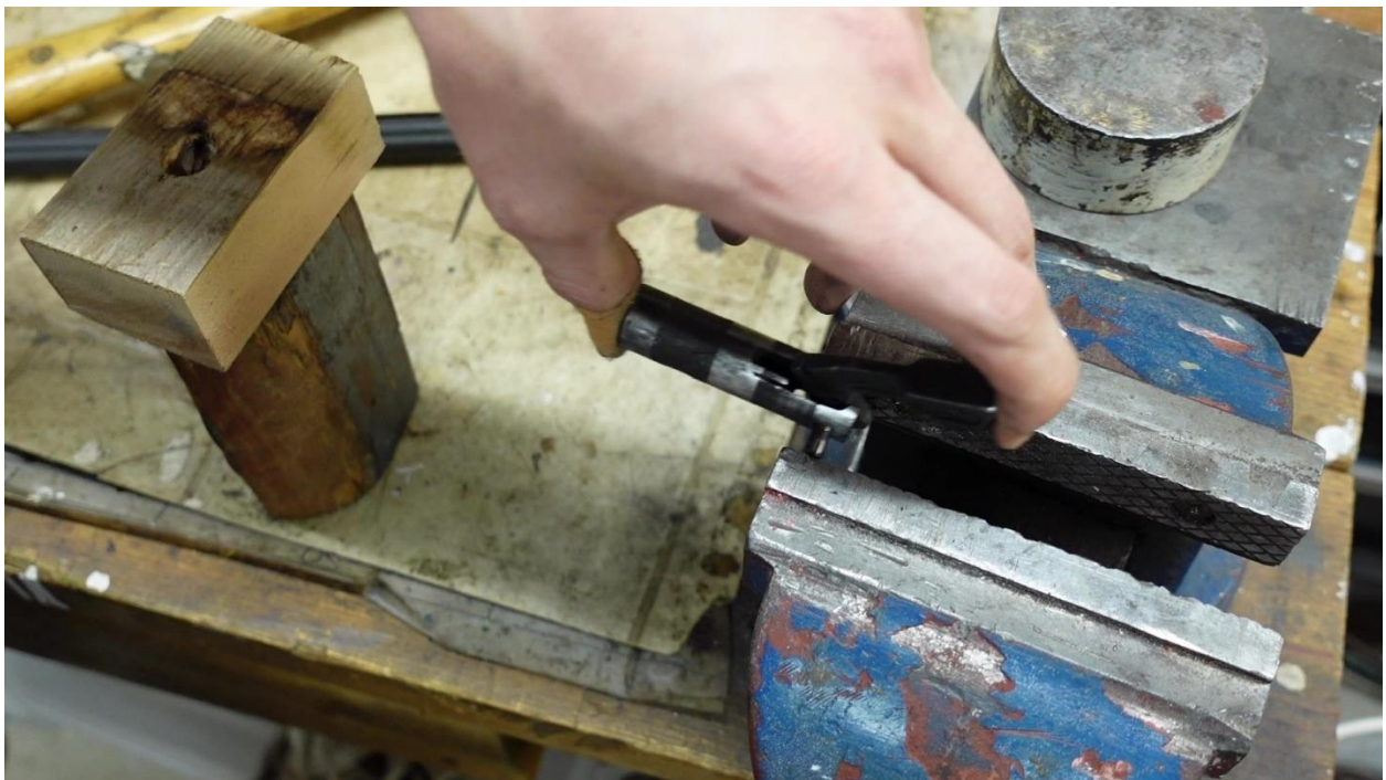
Re-install the pin – I used a vise to press the pin back into place. Make sure the pin hole is lined up!
