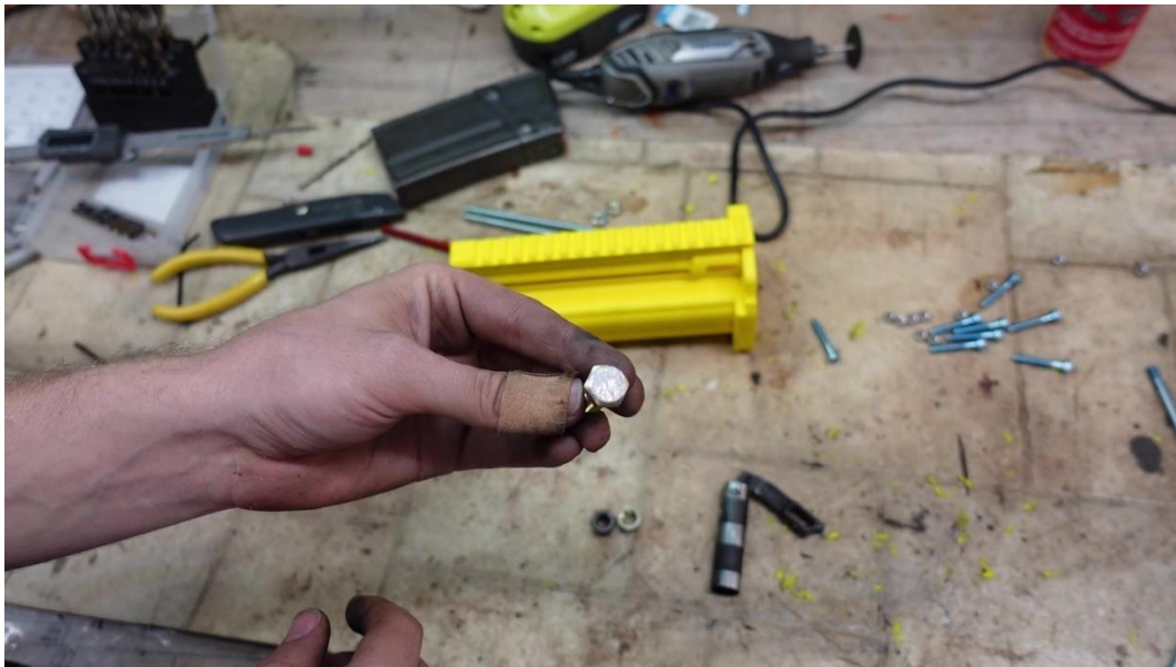
Use a Dremel tool or file to grind the face of the bolt smooth – remove any markings from the face of the bolt.
