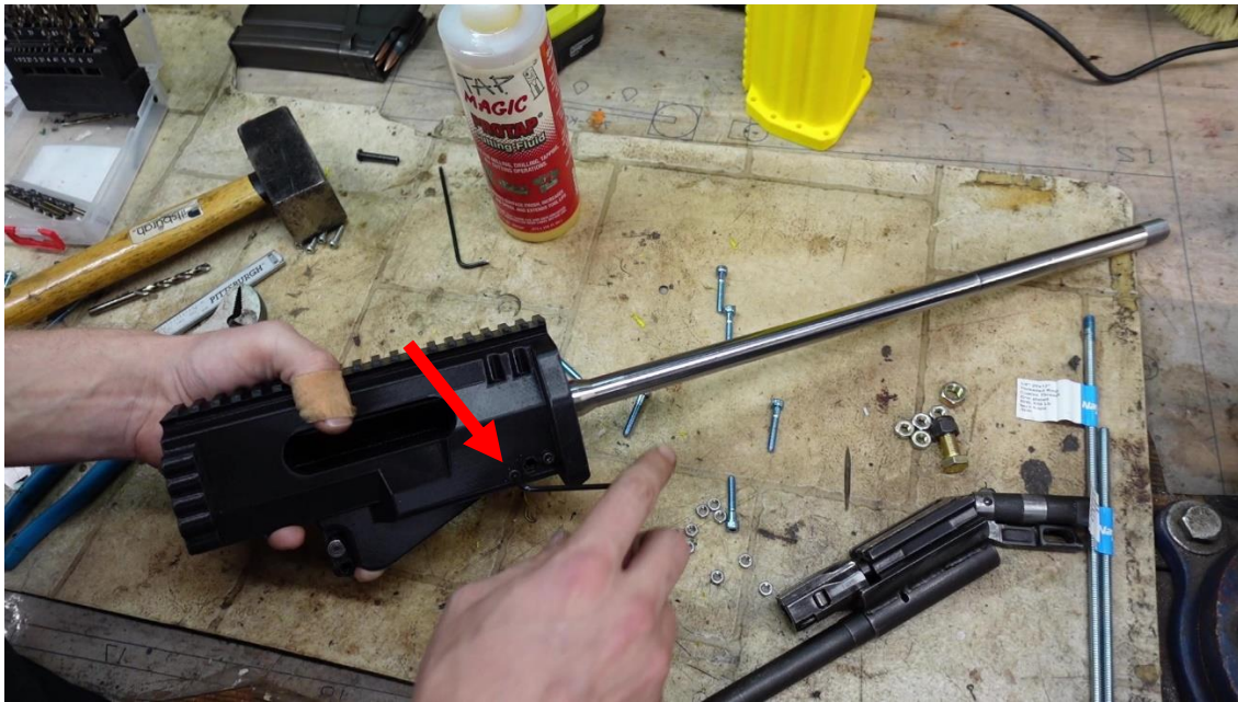
Installing one of the three M4x60mm bolts. Make sure you have a nut on the other side before you tighten your bolt down!
