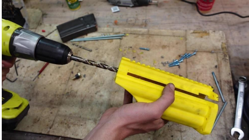
Drill out the hole in the front of the handguard with a 3/8" drill bit.
