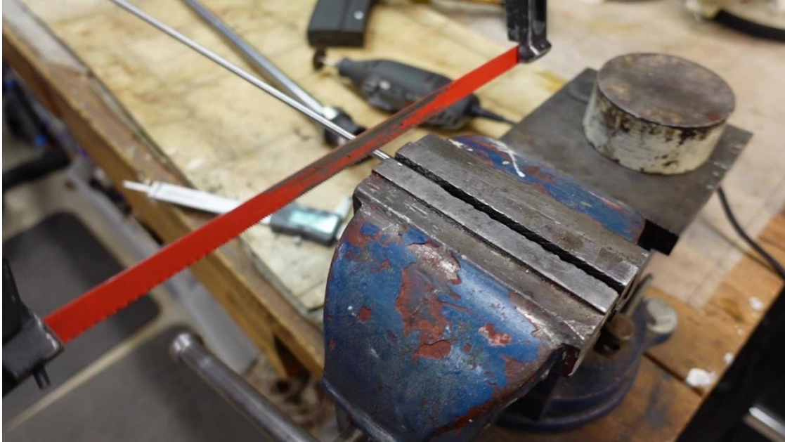
Cut your drill rod to length – these pins should be about 1" long.
