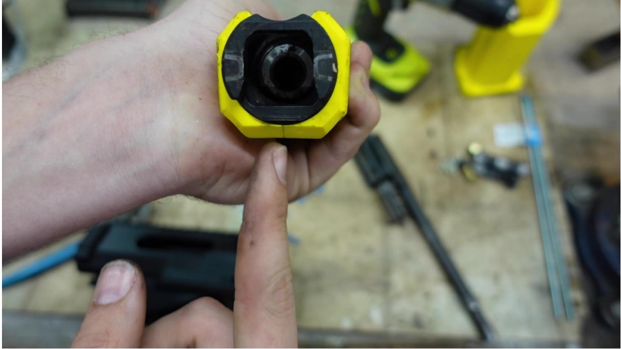
Align the seam where the two mounts meet at the bottom of the trunnion.
