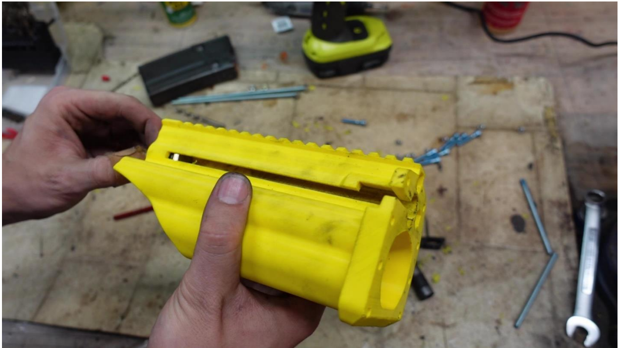
Line up the nut with the hex-shaped recess in the handguard, then pull it to seat it.
