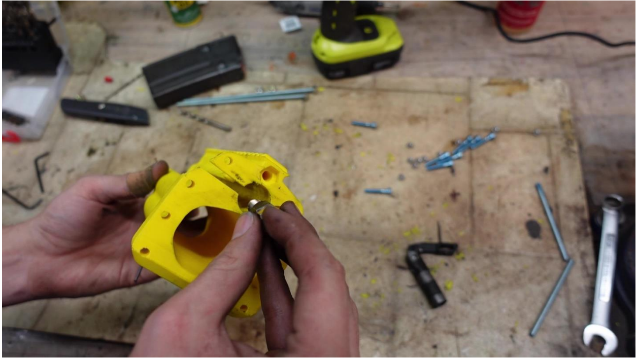
Drop the 3/8" bolt down the tube as shown.
