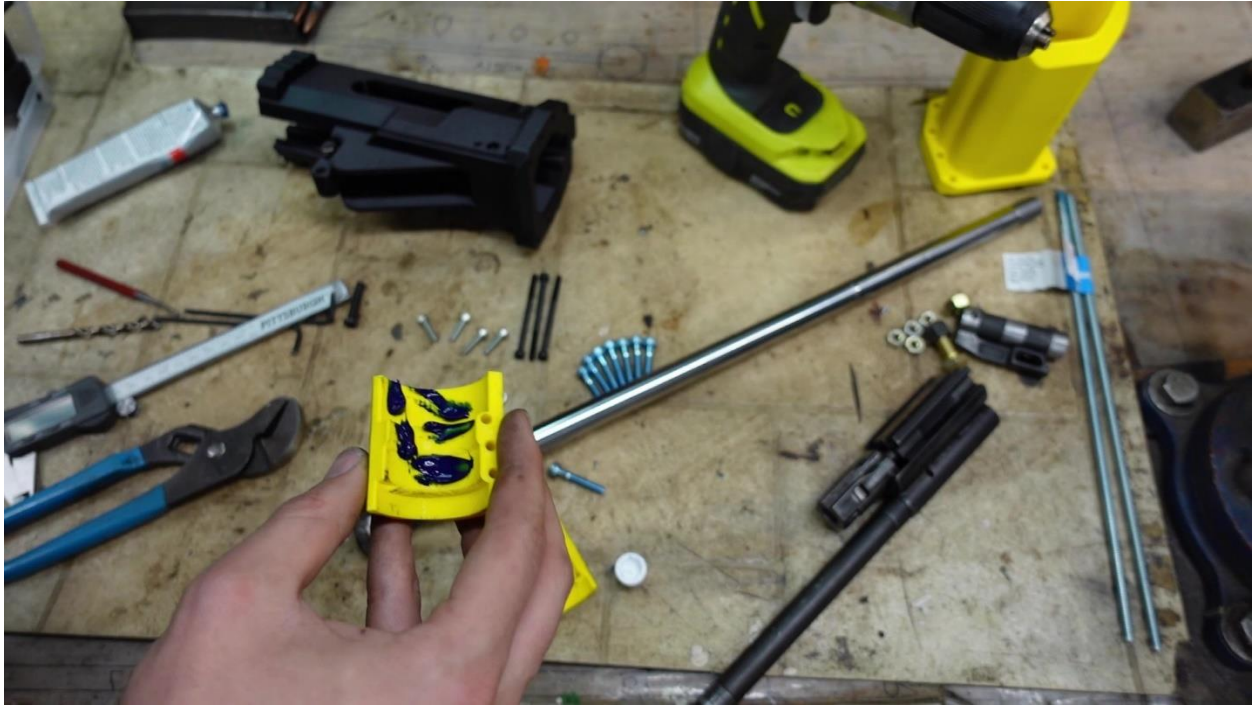
Apply some RTV to the mount.
