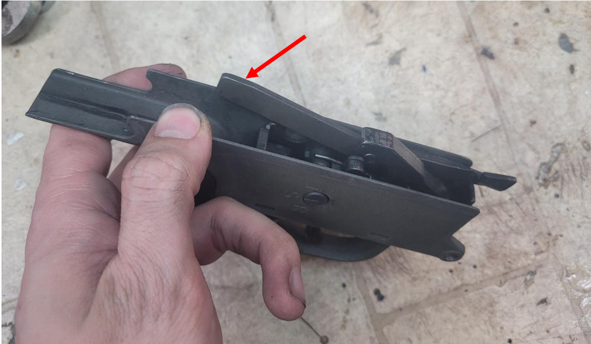
Where to lightly file to fix ejector-carrier hangups.
