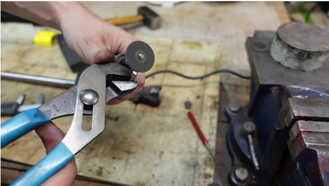
Adding a chamfer to the ends of the pin is a good idea.
