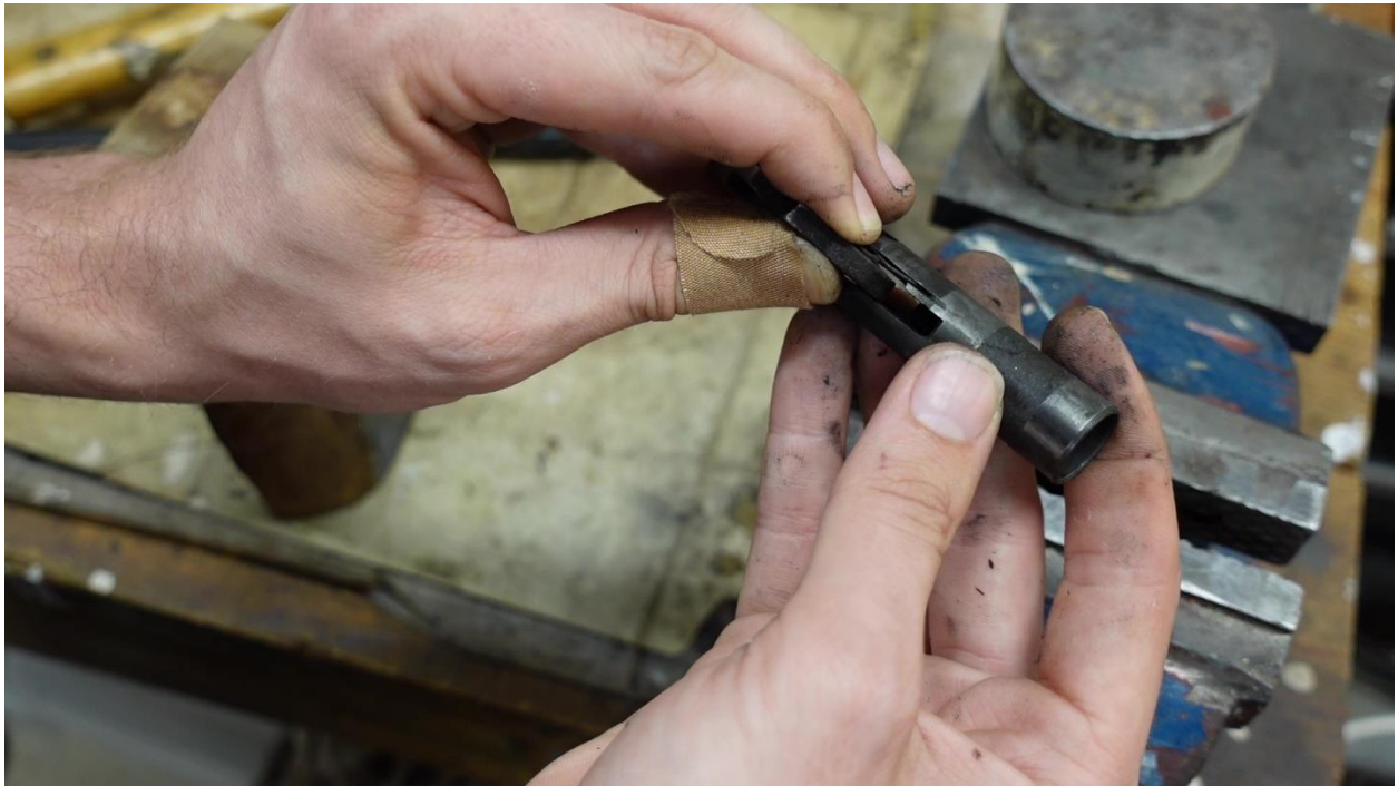
Correct position for the upper leg of the spring when installing the charging handle to the guide.
