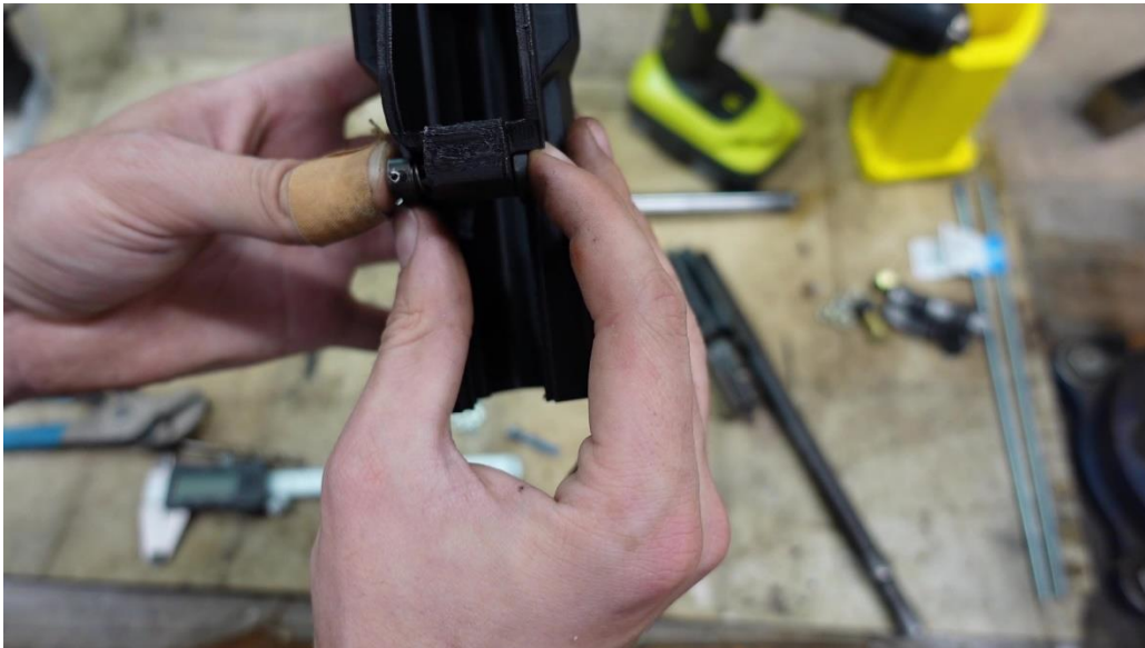
A view from the bottom of the receiver, showing how the button (on the left side) fits
