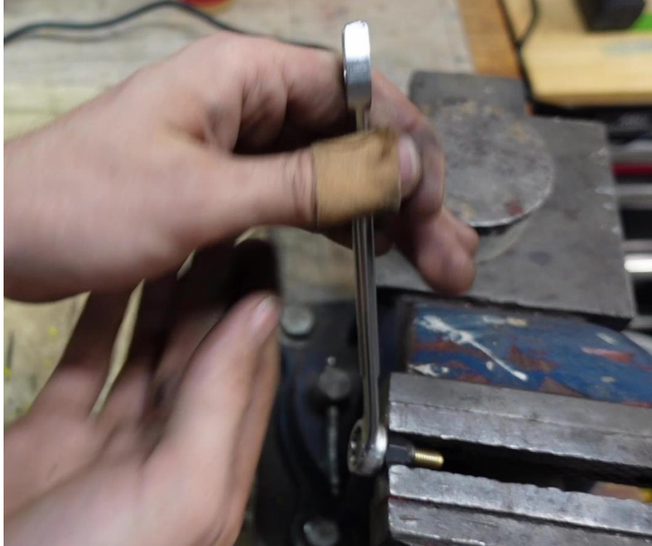
Thread the bolt fully into the locking nut.
