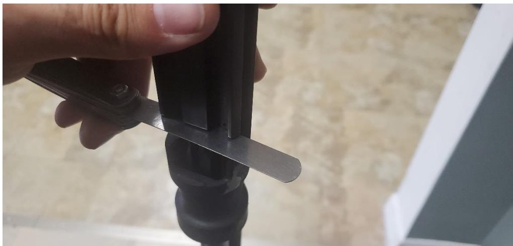
Where to measure bolt gap – between the bolt carrier body and the bolt head
