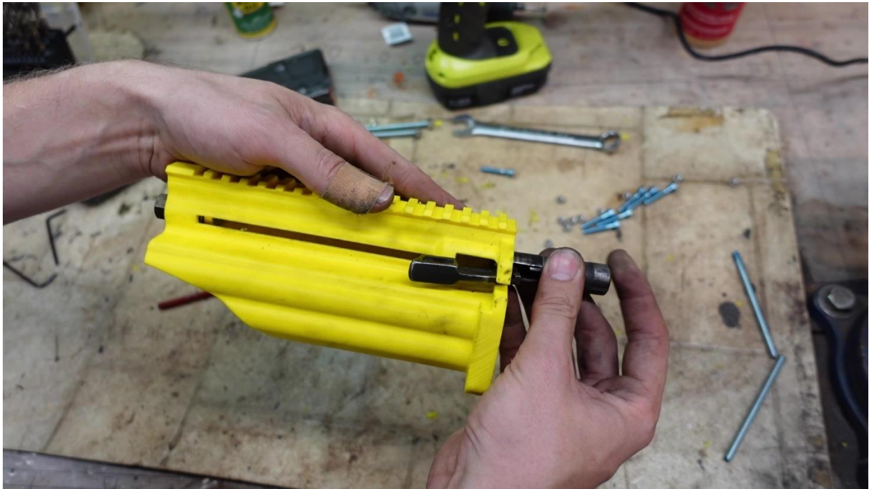
Slide the charging handle into the cutout in the handguard, aligning the guide with the tube in the handguard.
