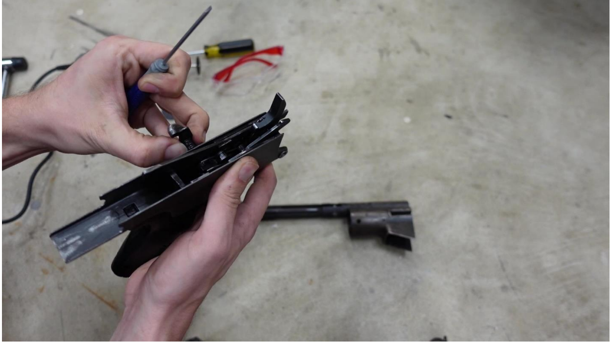
Pull selector out, paying attention if the selector is stuck on the tail of the disconnecter (seen above).
