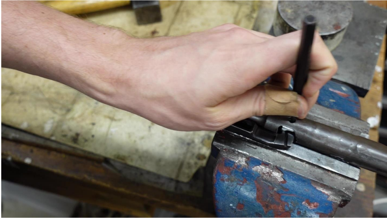
Punch the pin out using a punch
