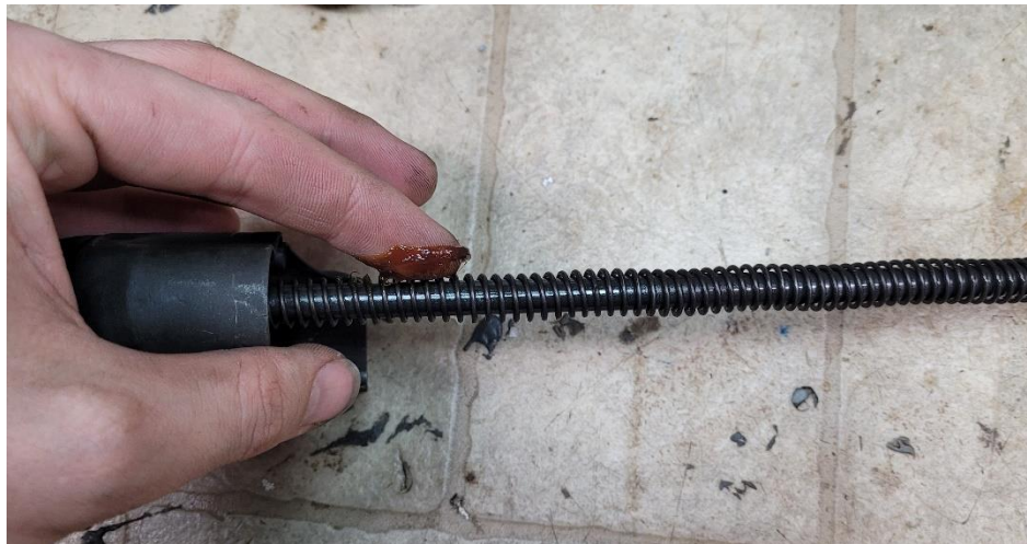
Apply plenty of grease to the recoil spring and guide rod to fix the recoil assembly-bolt hangups.
