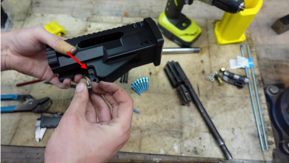
Magazine catch spring seated fully in its hole.
