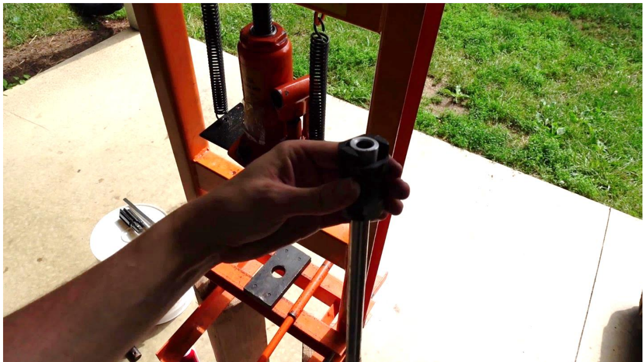
Place the barrel into the trunnion, muzzle first, from the rear end of the trunnion.
