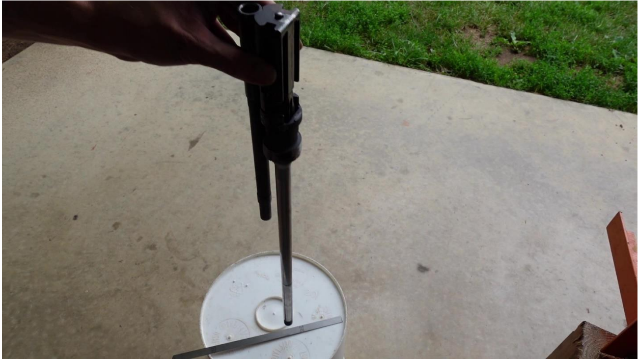
Hold the bolt carrier and trunnion assembly straight up and down before you measure bolt gap
