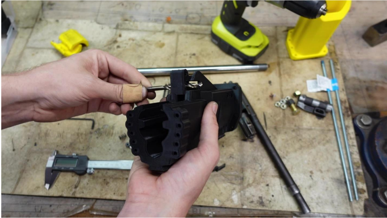
You may need to use a 6mm drill bit (spun by hand) to clean out the hole if the magazine catch feels tight
