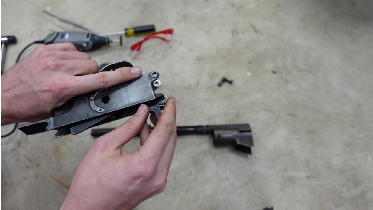
Pull the fire control unit out of the trigger housing by the hammer. You may have to wiggle it out.
