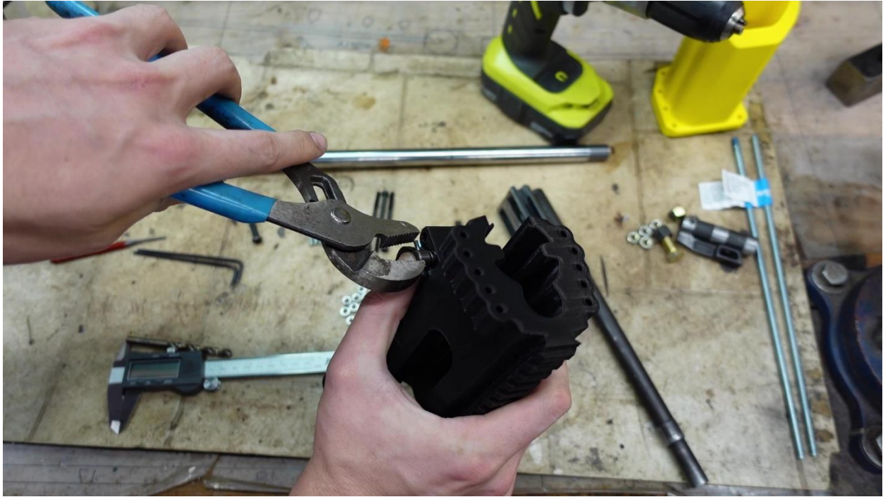
Make your setup look like this and squeeze with a pair of pliers to install the pin.
