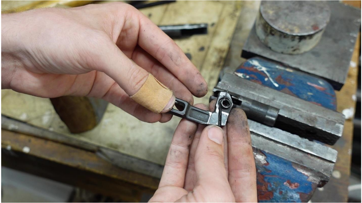
Correct orientation of the spring on the charging handle.
