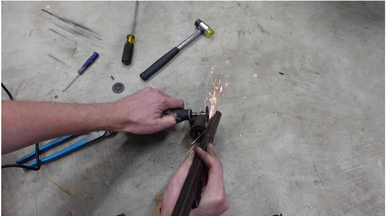
Cutting on the right side of the tube.
