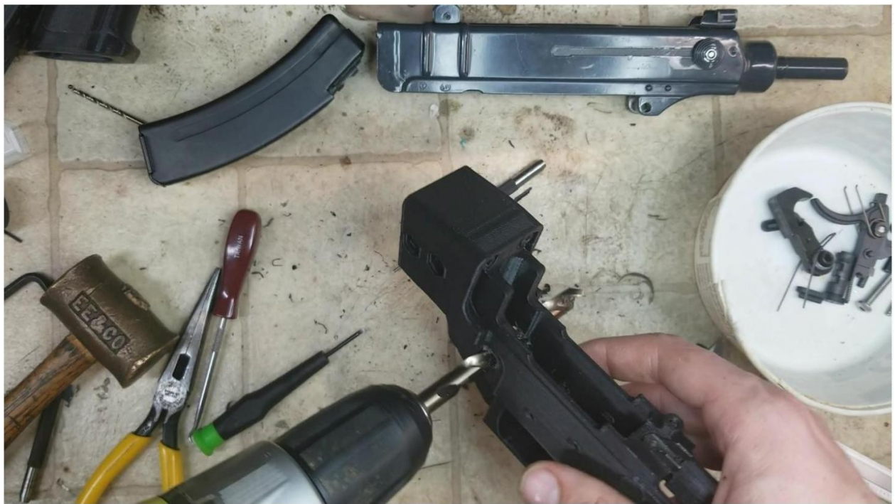
Drilling Selector Hole
