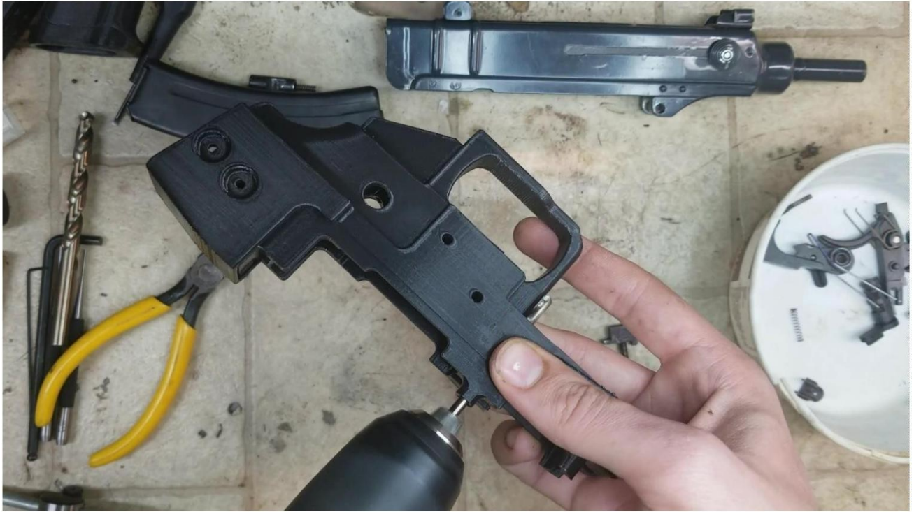
Bolt Catch Drilling
