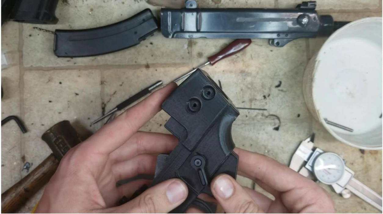
Installing Selector (Ensure it can Move Freely/Isn't Tight)
