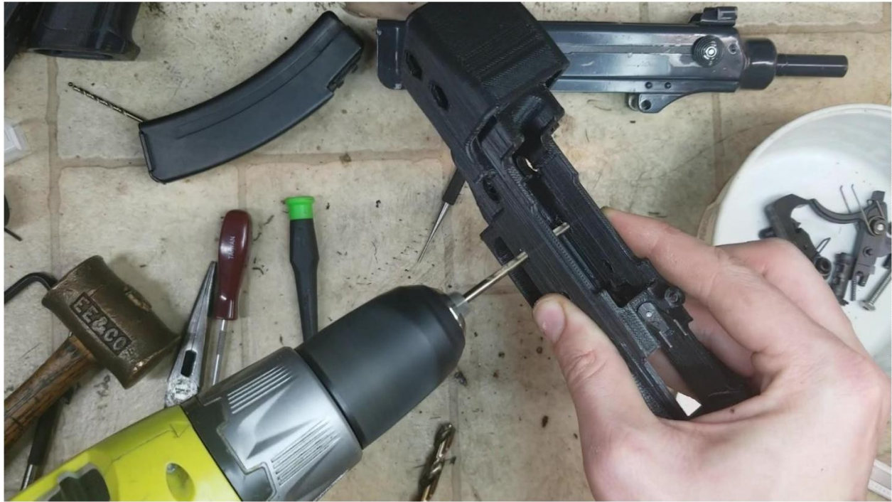
Drilling Fire Control Group Holes
