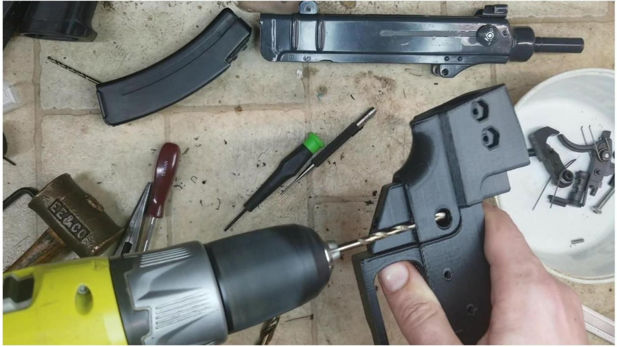
Drilling Selector Detent Hole
